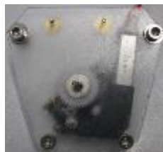
Figure 3: lock/ unlockA2 system: Flat motor
